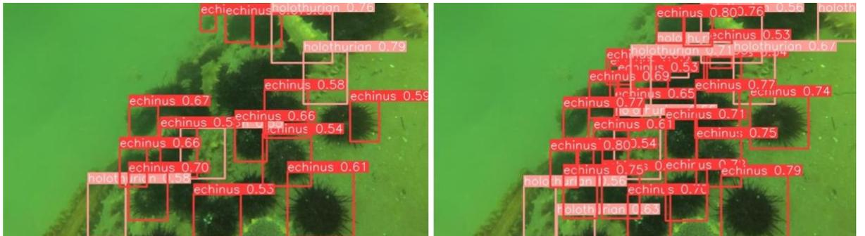
Fig 5. Image from the validation set processed by the baseline YOLOv8 (left) and our model (right). The number of misdetections of small dense objects decreased significantly.
